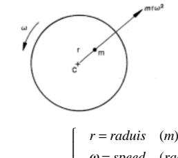
$$F = m * r * \omega^{2} where \begin{cases} r = raduis & (m) \\ \omega = speed & (rad/sec) \\ m = mass & (kg) \\ m * r = amount & (kg.m) \\ F = force & (N) \end{cases}$$
