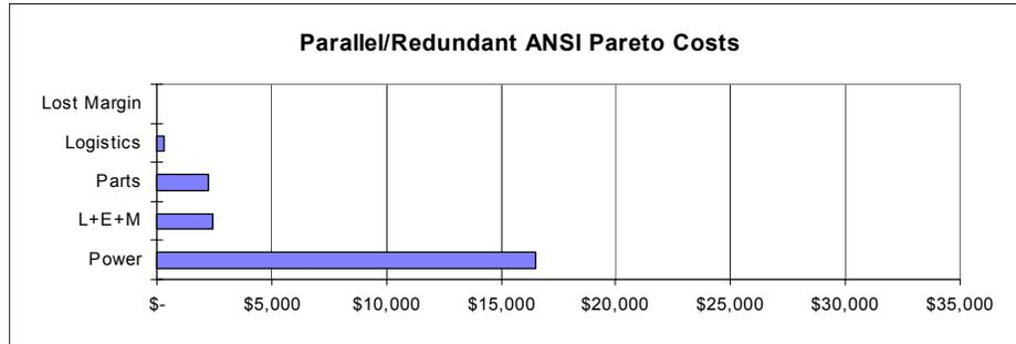
When redundant ANSI Pumps are installed, the Pareto chart looks substantially different as shown in Figure 7 where electrical power becomes the most significant cost item.
