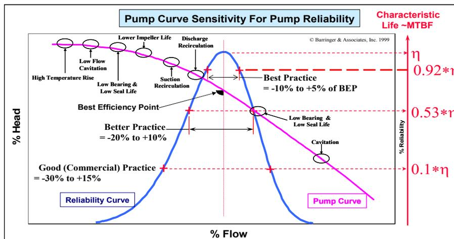
Figure 9: Pump Reliability vs Pump Curve
