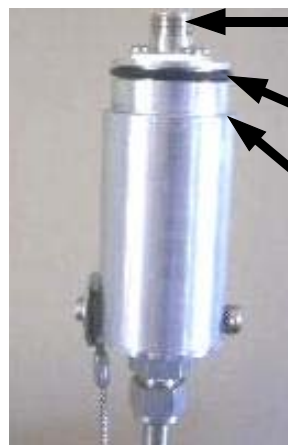
Figure 3. Probe for wet-well measurements, with either portable or fixed units.
