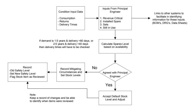
Process Flow used to Evaluate Sparing Levels
