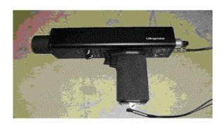
Figure 1 An airborne ultrasound instrument.
