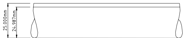
A 25mm SHAFT TOLERANCED TO h6 ISO TOLERANCE GRADE CAN BE AS BIG AS 25.000mm OR AS SMALL AS 24.987mm ON THE DIAMETER.
