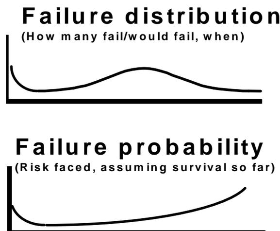
Figure 3. Failure Distributions vs. Underlying Probability Patterns
