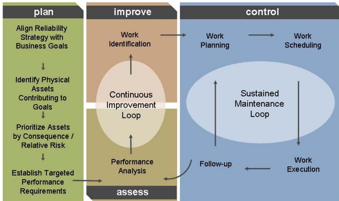
Figure 3: The Asset Reliability Process identifies what's required to manage the maintenance function.
