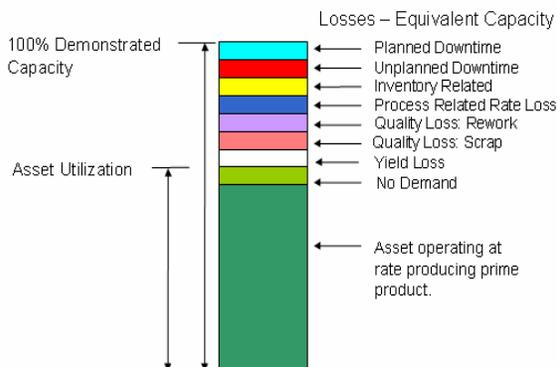
Figure 2: Asset Utilization is an example of a manufacturing level key performance indicator.
