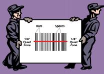
emitted from the laser scanner. But what's happening is that the scanner's light source is being absorbed by the dark bars and reflected by the light spaces. A device in the scanner takes the reflected light and converts it into an electrical signal.
