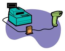
UNDECODED SCANNER CONNECTS TO BATCH OR WIRELESS TERMINAL
