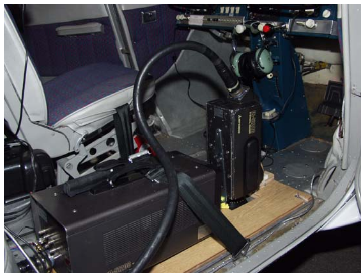
Figure 3) Large format infrared imager, fixed-mounted in a light aircraft.
